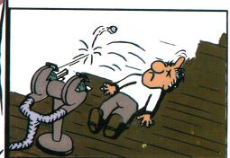
DON'T STAND DIRECTLY IN FRONT of a grinding wheel whenever a grinding wheel is started.
