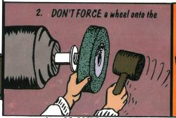
machine OR ALTER the size of the mounting hole--if wheel won't fit the machine, get one that will fit properly.
