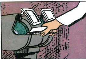
7. DO always USE SAFETY GUARD that covers a minimum of one-half, (1/2), the grinding wheel.
